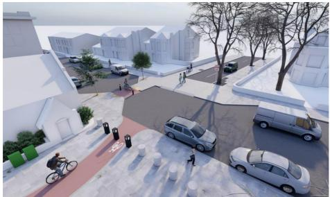
Figure 38. Modal filter and continuous footpath
