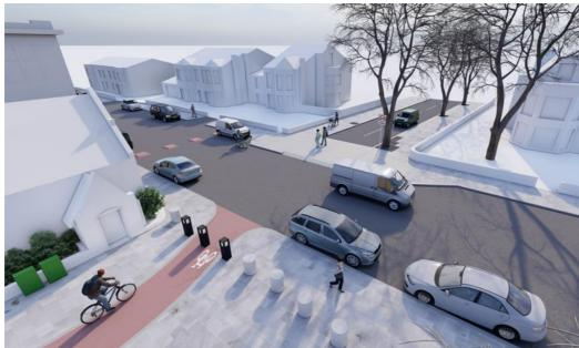
Figure 34. Continuous footpath along Hartington Road
