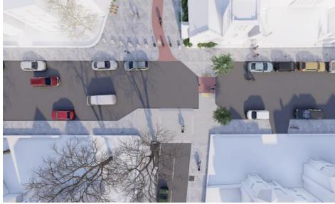
Figure 37. Bird's eye view of modal filter and continuous footpath
